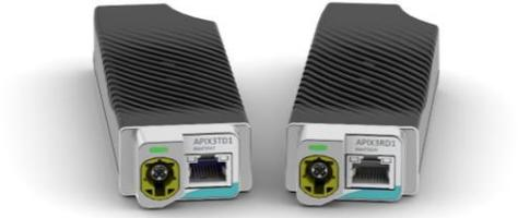
[Flexmedia XM APIX3RD1](#), based on INOVA INAP592R chipset, offers a frame grabber and real-time video stream analyzer for dual independent video stream analysis, performing BER/PER/PSN analysis. It provides a region-of-interest (ROI) multiple & simultaneous analysis with video timing detection and burst capable video frame grabbing. As for the generator, the analyzer as well supports bidirectional sideband communication.
