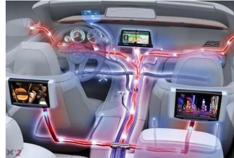
The third generation of APIX (APIX<sup>®</sup>3) is targeted to address the enhanced requirements for Infotainment and Cockpit architectures in vehicles. Those architectures support multiple automotive UHD resolutions in car displays based on the most recent and future generations of high performance SoC.
